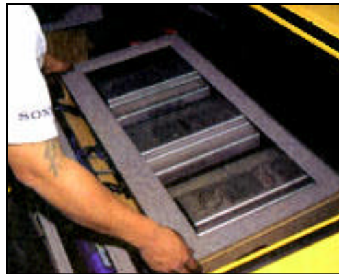
30 – To match the battery and CD changer with their tweed trim, a Masonite panel was used to frame the amps and the capacitors. These panels were, of course, covered in the same tweed.
