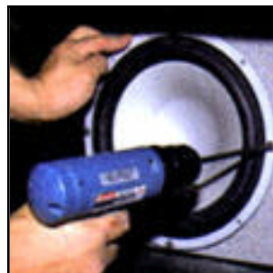
2 - Constructed from 3/4-inch MDF, the sub enclosure was designed to house four 10-inch Alumapro Alchemy subwoofers. These speakers were chosen not only because they create immense amounts of bass with almost no enclosure, but also for their aluminum cones. All of the speakers in the vehicle have aluminum cones and this blends nicely with the car's nearly all billet aluminum power plant and the Tube Driver amps.
