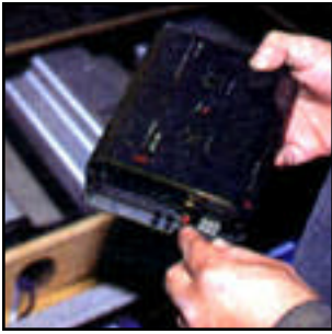
23 – A PPI 2-way electronic crossover was next on the bill. It was stashed just to the side of the amp rack so that it could be easily accessed for system tuning.
