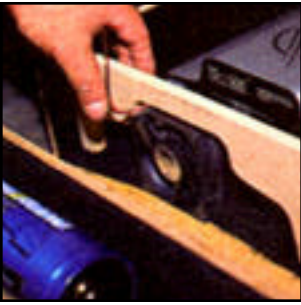
13 – For added ventilation, a couple of fans were installed in each side of the amp rack in a push-pull configuration. This way heat drawn out of the amp rack and cool air directed in.
