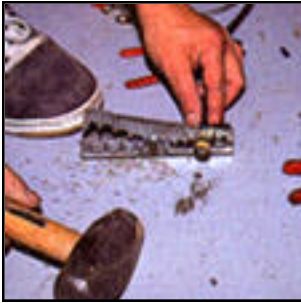
11 – Several of the larger-gauge cables were terminated with gold connectors from Lightning Audio. These larger terminals require a special crimp tool to insure a long-lasting union.
