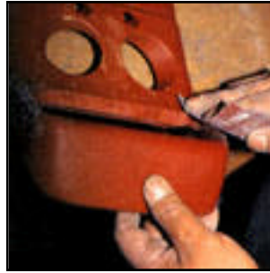
18. The body filler then was shaped to match the contour of the console and then sanded smooth.
