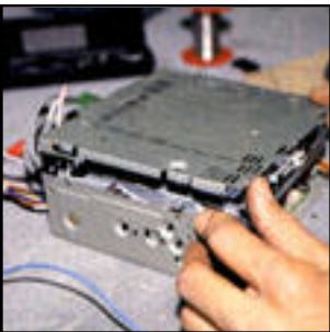
14. Next in line was the source unit install. First, the Pioneer source was gently dismantled.
