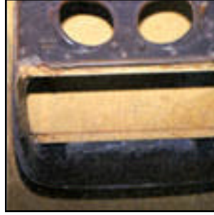
17. Next, the console had to be modified to house the faceplate that was substantially wider. To do this Mike fiberglassed a few pieces of Masonite to the top and bottom to the opening and cut-back the sides. Fiberglass reinforced body filler was then applied to the necessary areas.
