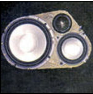
13. With the pods completed and covered in black carpet that matched the car, the Tube Driver speakers were wired up and dropped in place. All that the Xtreme Audio crew had to do next was fabricate a set of grilles and the front stage was in business!
