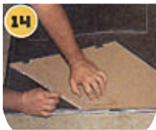
14 & 15 – Even the C-pillars got the VB-2 treatment. We used the VB-2 on any accessible panel that had the potential to transmit noise into the car.
