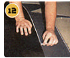
12 & 13 – Just as with the door panels, we were able to use existing interior panels to determine the shapes for our VB-2. This piece will fit perfectly on the rear package tray.
