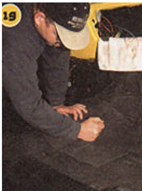
19 – A good pounding helps form the lead to the floor panels.
